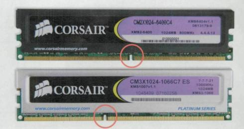
**KEYED FOR YOUR PROTECTION** The top module is a Corsair DDR2 module; the bottom one, a DDR3. Note the different locations of the key notch in each edge connector.
