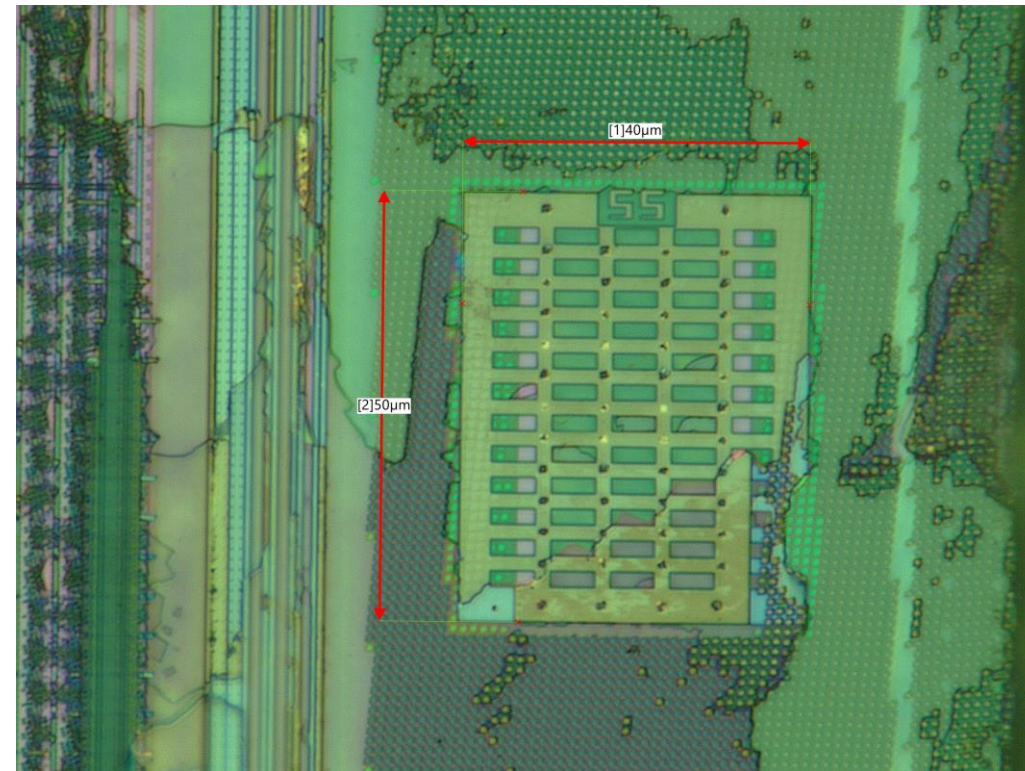
Die edge test pads for pre-stacking wafer probe test
