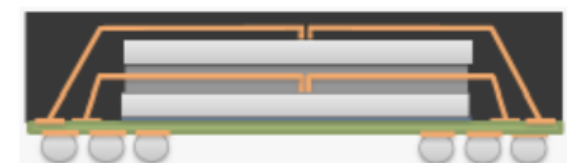
Without RDL on top die Cons: Au wire cost, signal integrity issue
