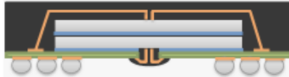
Without RDL on top die Cons: Au wire cost, signal integrity issue
