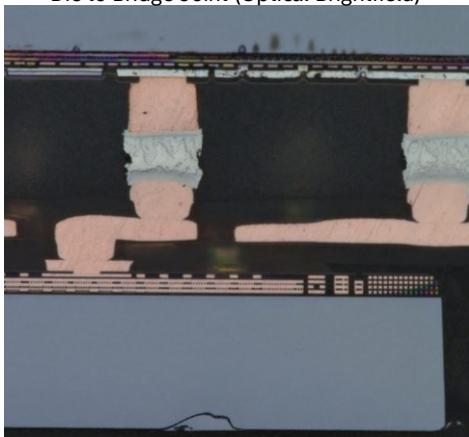
Die to Bridge Joint (Optical Brightfield)
