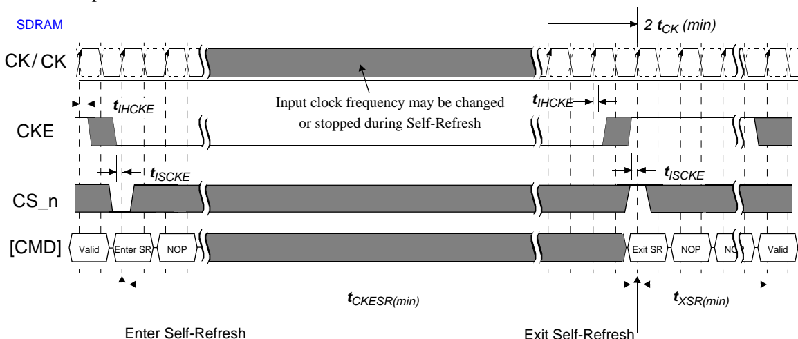
Figure 77 — LPDDR2-SX: Self-Refresh Operation
