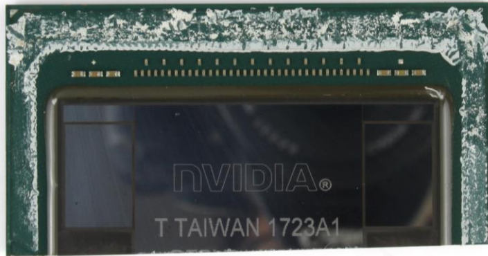
Package Top View – Metal Frame Removed ©2018 by System Plus Consulting
