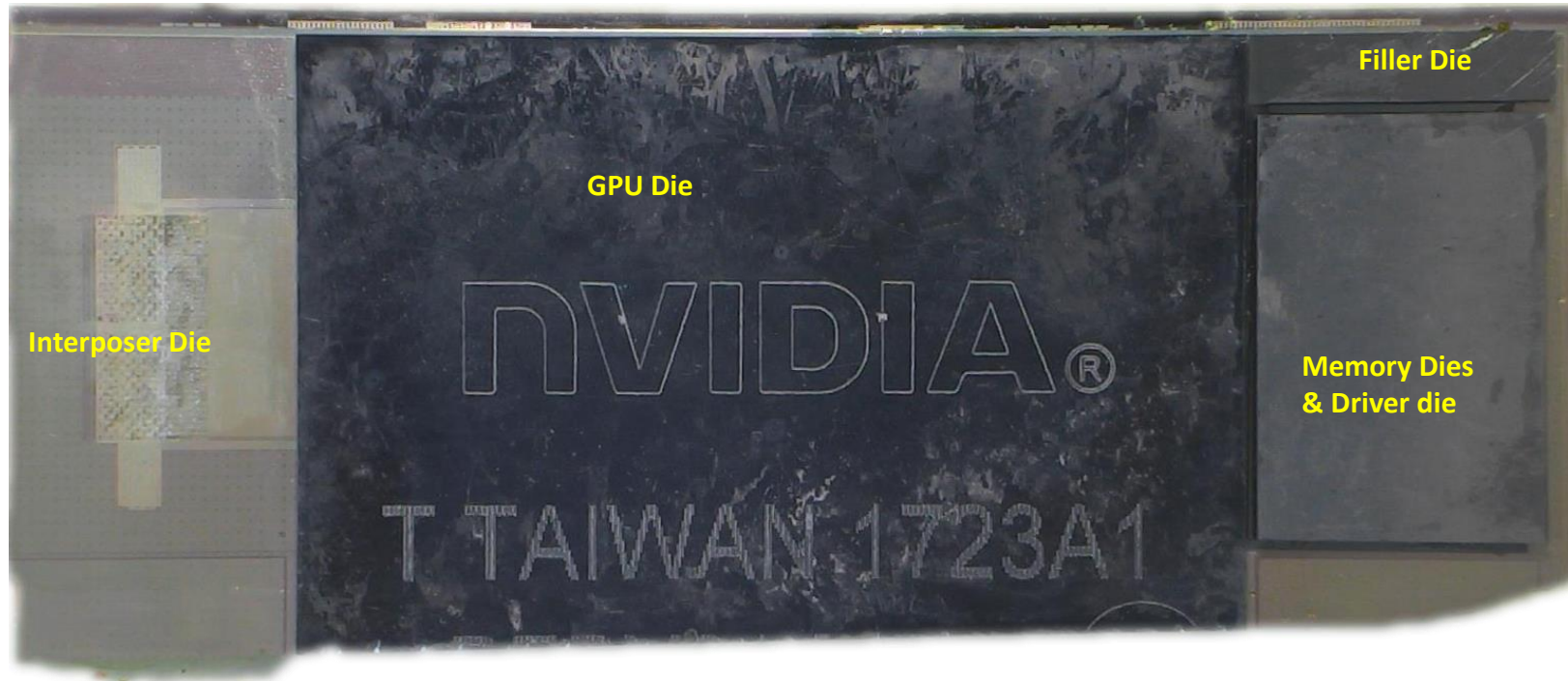
Package Top View – Underfill removed and Right HBM Memory Removed ©2018 by System Plus Consulting
