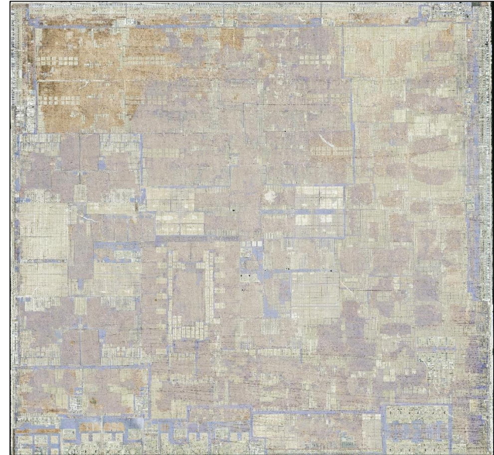
Die Overview after removing of the metal Layers ©2020 by System Plus Consulting
