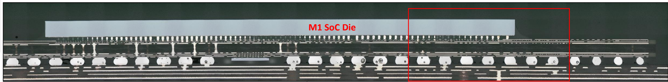
M1 SoC Package Cross Section ©2020 by System Plus Consulting
