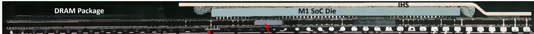
M1 SoC Package Cross Section 1 ©2020 by System Plus Consulting
