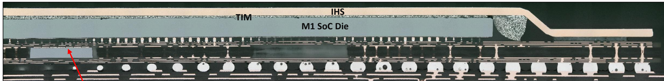
M1 SoC Package Cross Section 1 ©2020 by System Plus Consulting
