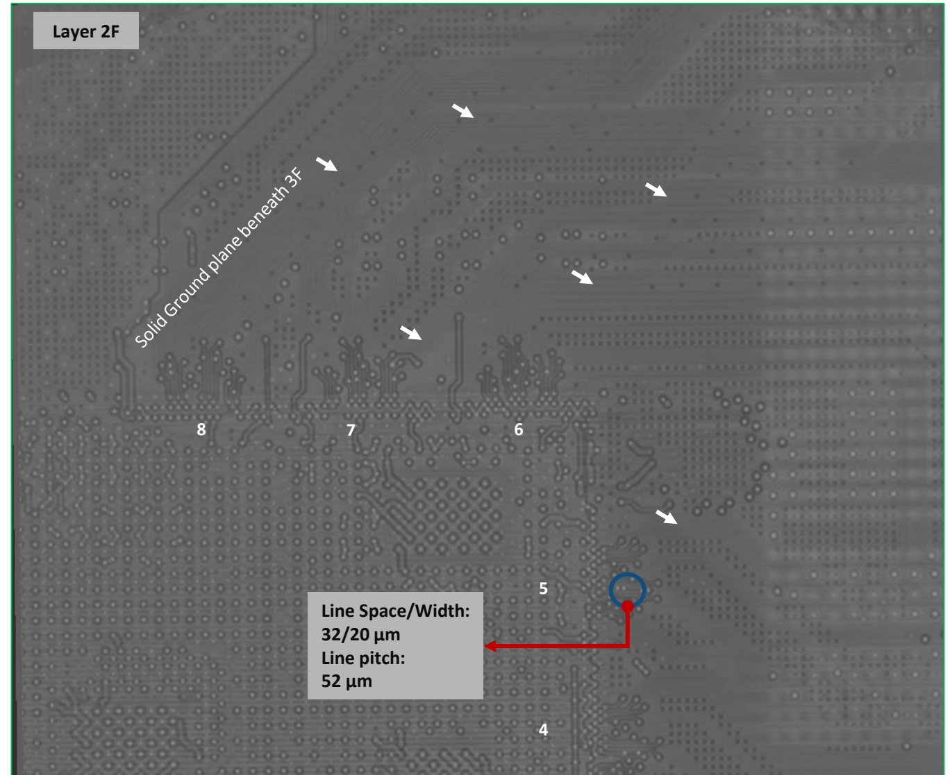
PCB Substrate Layer 2F – X-Ray View
