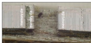
Memory Package Opening (after metal wire removal) ©2022 by System Plus Consulting
