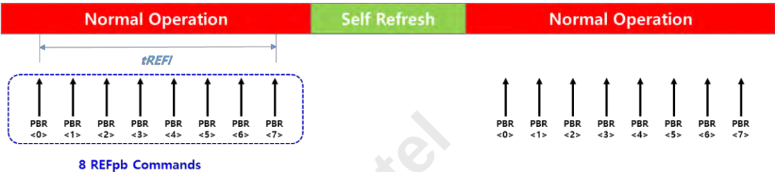
Figure 141 — Optimized Refresh Operation Example for REFpb (Completion of the Bank Count by 8 REFpb Commands)
