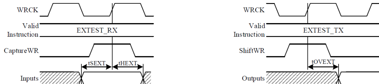
Figure 112 — IEEE1500 EXTEST_RX and EXTEST_TX Instruction Related Timings
