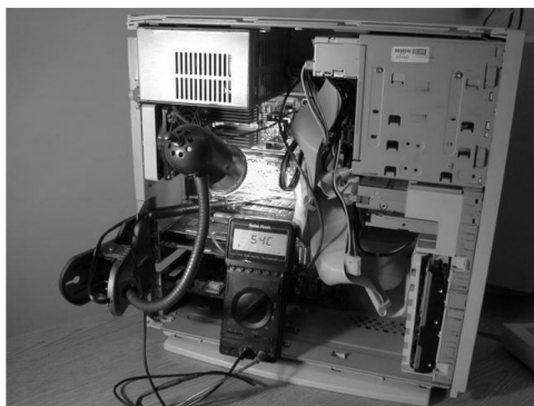
Figure 3. Experimental setup to induce memory errors, showing a PC built from surplus components, clip-on gooseneck lamp, 50-watt spotlight bulb, and digital thermometer. Not shown is the variable AC power supply for the lamp.
