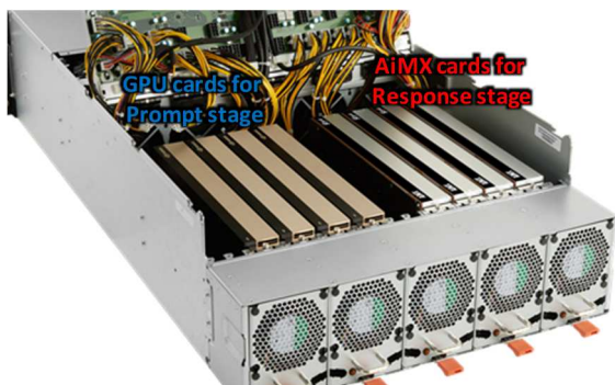
Fig. 7. Prototype inference system using GPU and AiMX cards.
