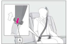
2 Insert the mechanical key  $(\rightarrow P.88)$ or plate B into the notch of buckle and remove the belt.
