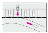
When the distance between your vehicle and metal objects, such as a guardrail, wall, sigh, or parked vehicle, which may reflect electrical waves toward the rear of the vehicle, is short 4
