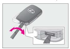
3 Remove the depleted battery.
