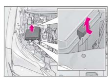
► Engine compartment: type B fuse box
