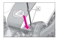
5 Holding a rag under the end, pull the dipstick out and check the oil
