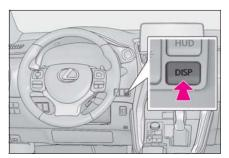
Until the screen changes, continue pressing the "DISP" button, and it will repeat until the item desired to be changed is displayed. Customization can be performed when the head-up display is on.
