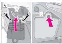
9 Install the engine compartment cover. (→P.320)
