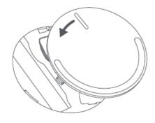
2. Place two AAA batteries into the battery compartment.
