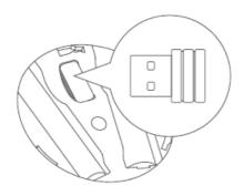
4. Insert the USB receiver into the computer's USB port.
